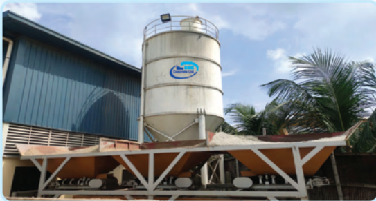
Block Silo & Material Bin
